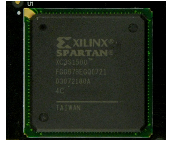
Figure 10. Xilinx Spartan-3 FPGA (XC3S1500-4FG676C).
